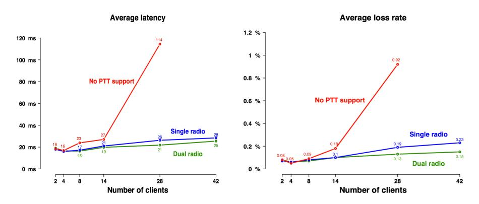
Average latency of the packets received by the mesh nodes, while increasing the number of clients on a single PTT group.
